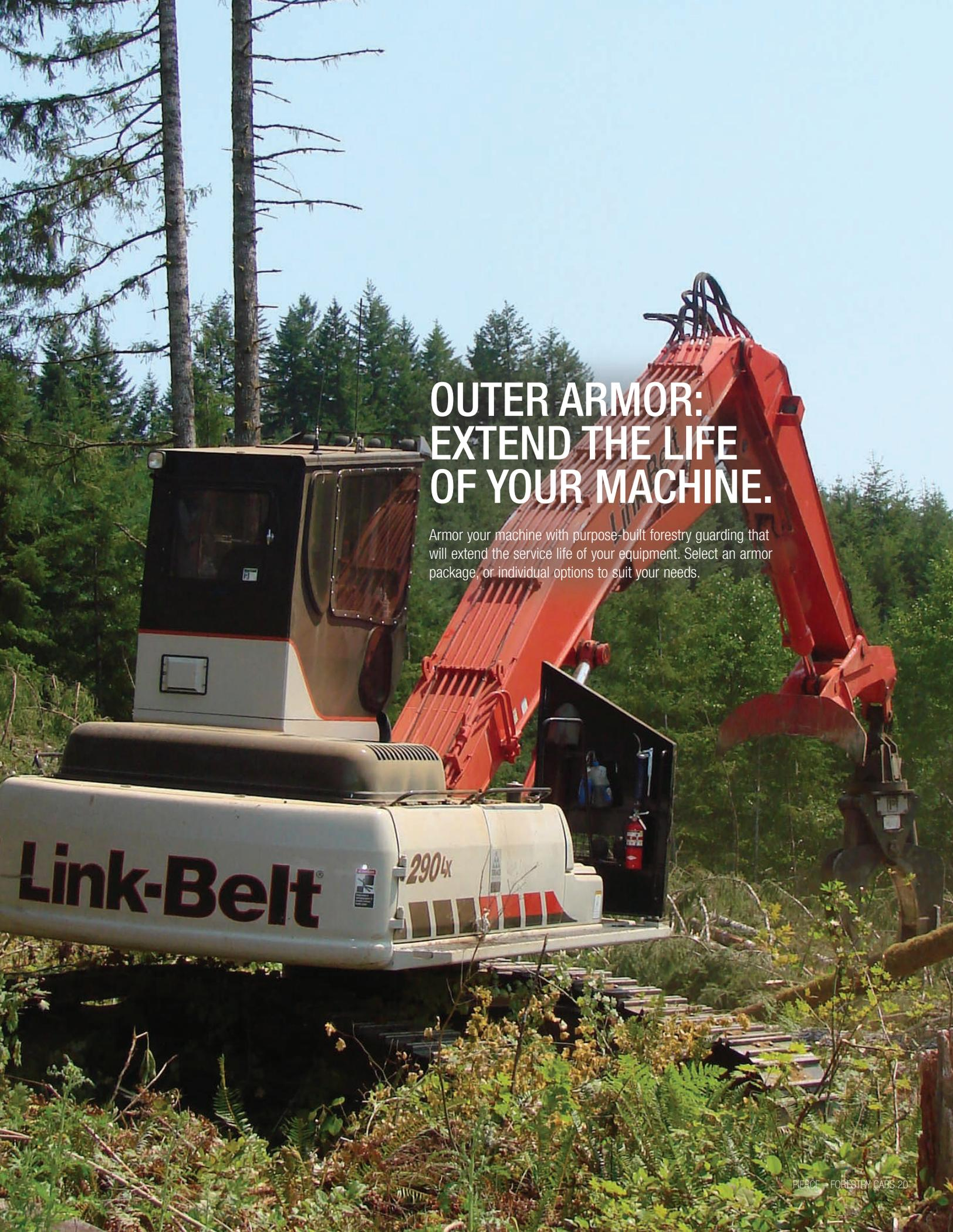
A Link-Belt 290LX excavator is shown in a forest setting. The machine is white with a red boom and bucket. It features a large, protective metal cage (forestry guarding) over the cab and engine area. The excavator is positioned on a log skid trail, surrounded by dense green forest. The background shows tall evergreen trees under a clear blue sky.
