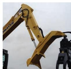
HEEL RACK (ATTACHES TO EXCAVATOR STICK)
