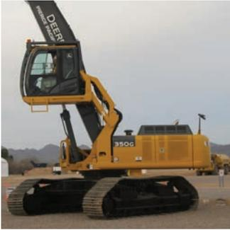
HYDRAULIC ELEVATING CAB
